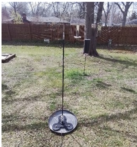
Figure 1 The "Garbage" antenna - a 20m hamstick on top of a metal garbage can lid.
